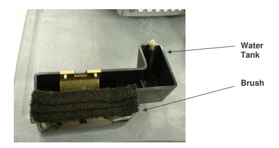
3. <u>Fill bottle with water</u> and place bottle on brackets on the side of machine. The spout of the tank will fit into tank reservoir.
