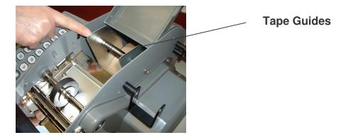
The tape roll guides should be properly set for the width of the tape being dispensed. The roll of tape should be center in the basket area and the roll guides adjusted loosely by lifting them and setting them on the desired pre-cut areas.
