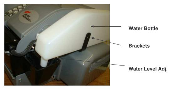
The <u>amount of water</u> required for proper moistening of different grades and types of tape will differ. Heavier adhesives or reinforced tapes will normally require a high water level. Lighter tapes require less water and a lower level.
